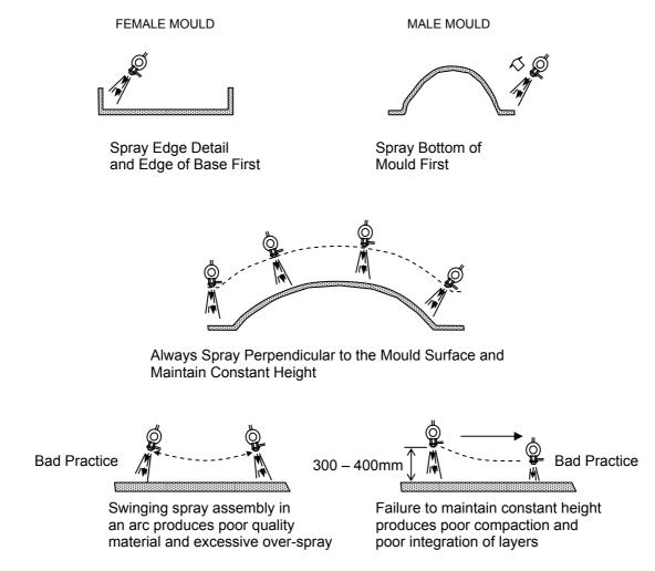
Some manufacturers prefer to introduce two rovings into the gun, and increase the slurry output to achieve a higher output. In this case the gun may be held further from the mould and the spray pattern adjusted changing the atomising pressure.
