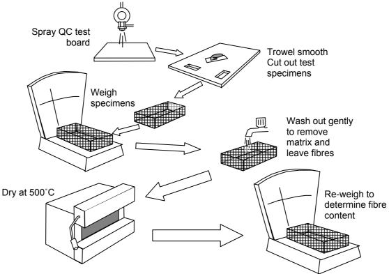
Procedure for determination of fibre content
