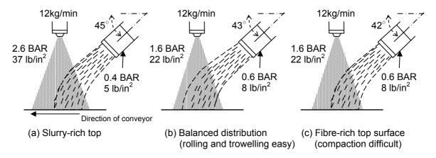
Illustration of Effect of Atomising Pressure and Angle of Deposition.
