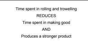
Compaction is required to:-
