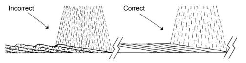
Higher cross-head speeds may be desirable when producing thin and narrow products at a high slurry output. However the inertia of the cross-head itself means that this is not always possible. Therefore, in these cases it is usually necessary to reduce slurry output and conveyor speed to achieve the same result.
