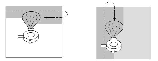
Schematic illustration showing 50% overlap of layers
