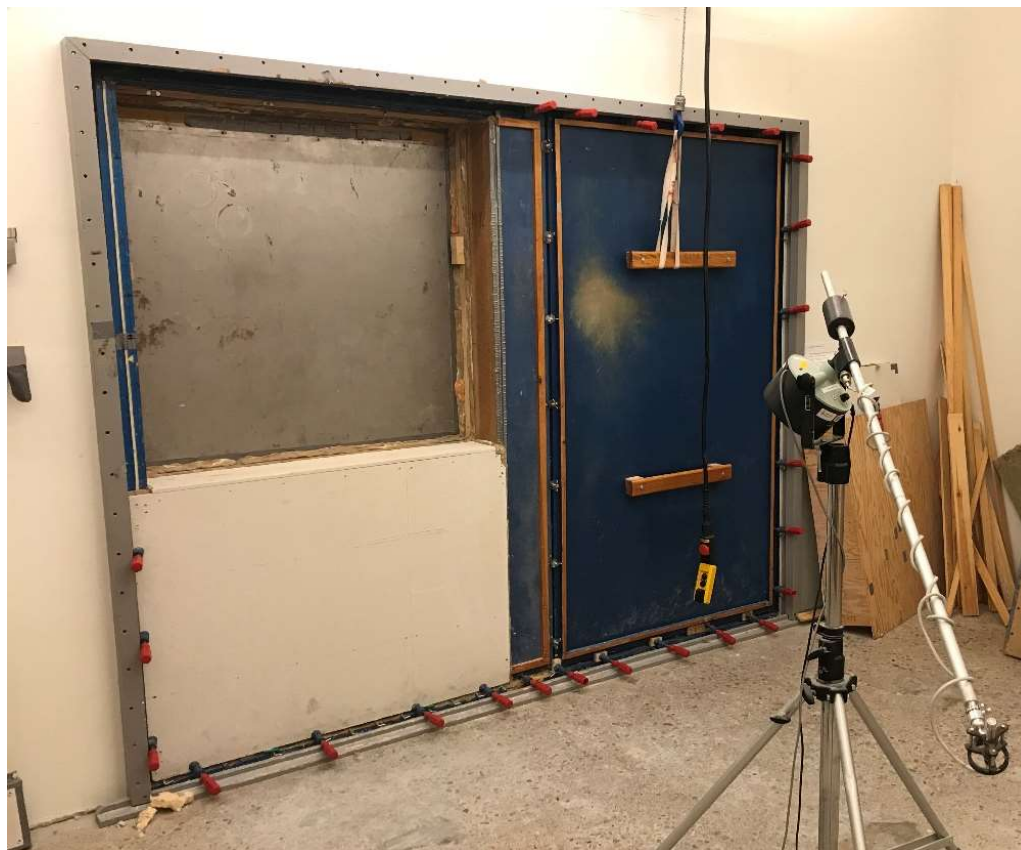
Figure 1: The quadratic steel-plate clad wooden frame in the variable test opening, as seen from the sending room at the time of mounting.
