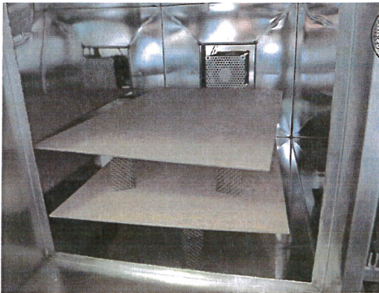
Figure 2: Test specimens in the 230L emission test chamber.
